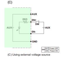
\*GND shown in above diagram is referring to the GND of CN2, not the Grounding from main power(NEG-).\*
